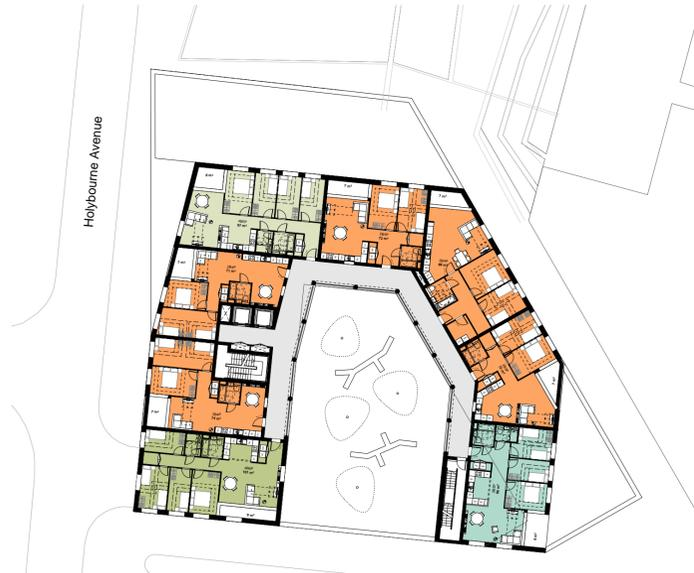
BLOCK A - Typical Upper Floor Plan
